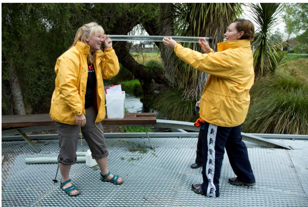
Figure 2.7: SLLT volunteers measuring clarity using a clarity tube at Smacks Creek. The volunteer on the left is looking through the tube for the black disc which the volunteer on the right is moving down the tube.
