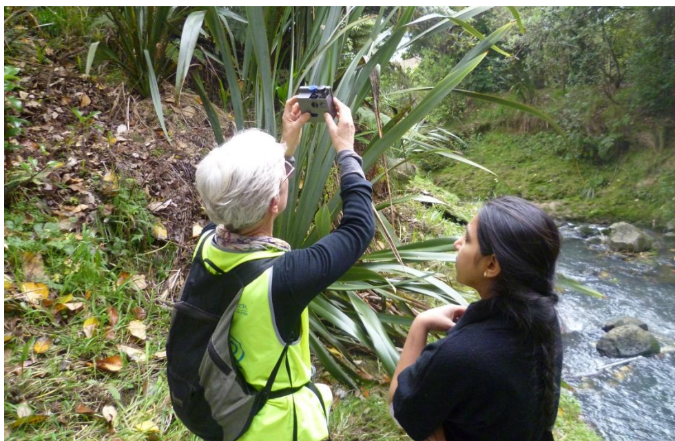
Figure 2.8: Wai Care volunteers measure DO by comparing the sample with a coloured wheel denoting different concentrations of DO. This site is at the Unitech Bridge.
