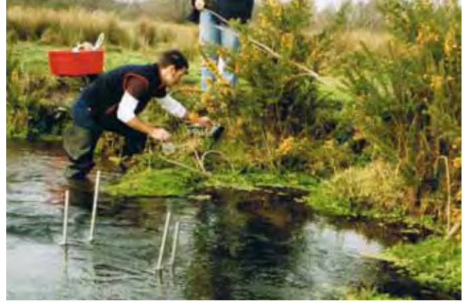
Figure 3b. Field measurement of IGDO. Two readings were recorded from water samples taken from two depths at each of two trout redds. The YSI® DO meter is in the foreground.
