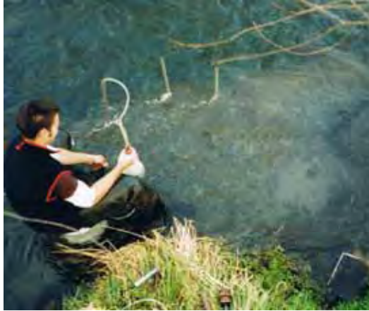
Figure 3a. Pumping water samples from stainless wells driven into a trout redd.
